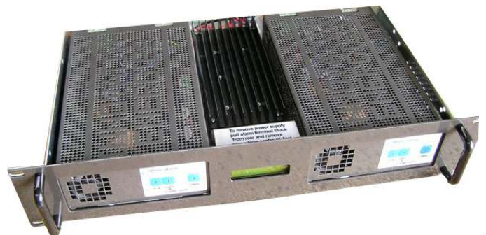
2U rack with 2 x SR250D12 power supplies and decoupling diodes on heatsink plus V/I meter
